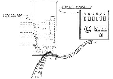
4. Insert the wires from the flex conduit up through the knockout; take care to not nick or gouge the wires on the metal edge. Tighten the locknut securely onto the load center. The wires can hang freely.
