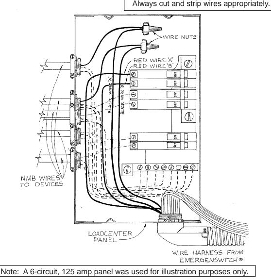
9. These steps are continued for each desired circuit (keeping in mind that if the circuit is a GFCI circuit breaker, it will not be a GFCI circuit while it is powered by the generator). In the event that a 240 volt (2 pole) circuit will be used, the same concept is used.
